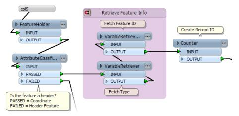
The next section of workspace checks for the end-of-feature marker, then creates a point for each coordinate pair. Remember, each line has two coordinate pairs on it — one is flagged A and the other B.
