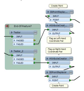
The final part of the workspace sorts the point features into order, turns them into the final geometry, and finally writes the output to Geodatabase:
