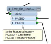
Where the workspace deals with headers is an AttributeClassifier transformer. It tests to see whether col0 is a numeric value (i.e. test = Not Header).
